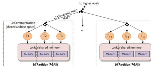
These Worker nodes correspond to the partitions of the HPC application. Each Worker node is an entire sub-system including processing units, memory, and storage. Within a PGAS domain (consisting of several Workers), the proposed architecture offers a shared partitioned global address space and shared partitioned reconfigurable resources that can be accessed via regular load and store instructions without using any global cache coherent mechanism.
